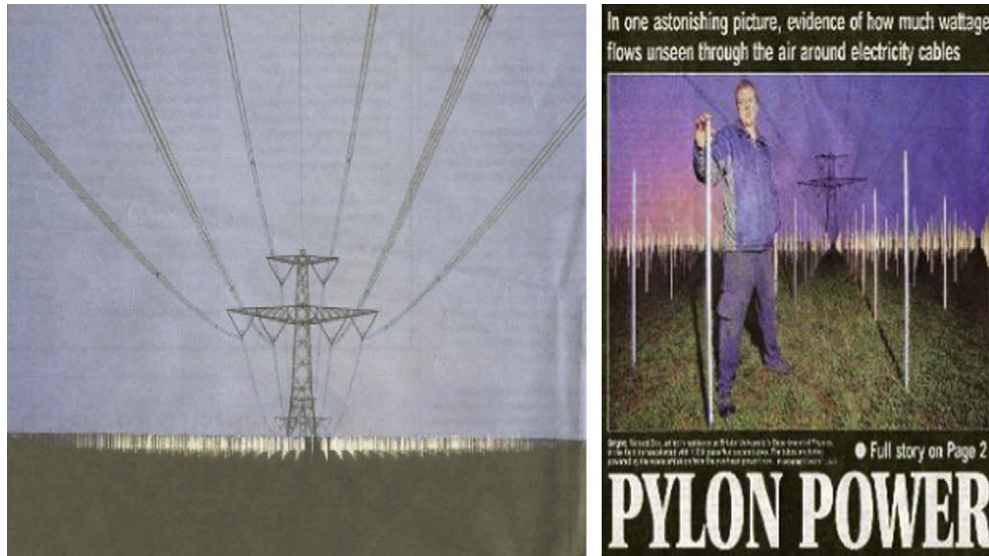
Fig. 7. "Invisible" electricity made visible by fluorescent tubes. (Source: Evening Post, UK, 19 February 2004, p. 1.)
