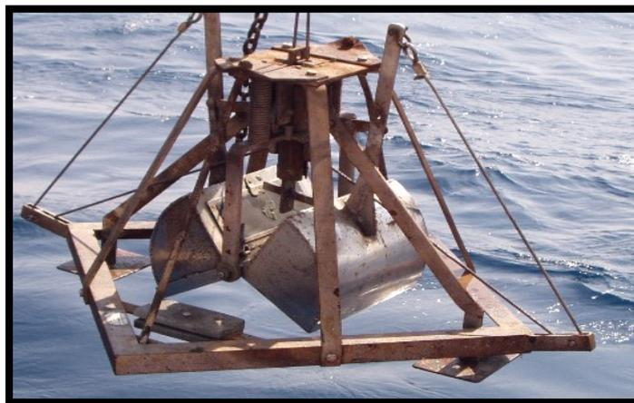
**Fig.2. Smith-McIntyre Grab sampler (Photo courtesy: CMLRE)**
